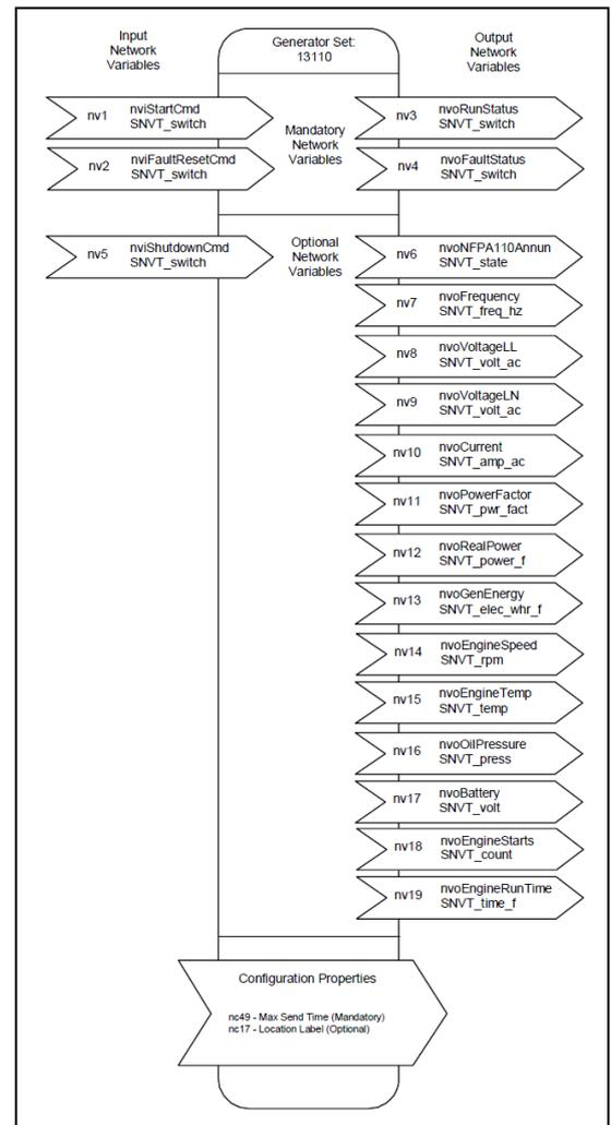
Figure 2. Generator Set functional profile.
